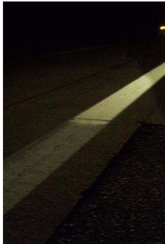
Cross point border marking Paint / CP Agglomerate on freeway A 2 at night, direction Hannover, km 12,5
