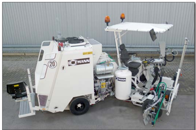
Narrow and extremely manoeuvra- ble machine with laterally adjustable cockpit to the right side, therefore ...
