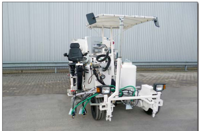
Narrow and extremely manoeuvra- ble machine with laterally adjustable cockpit to the right side, therefore ...
