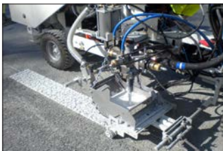
... screed box system (not path-dependent)
