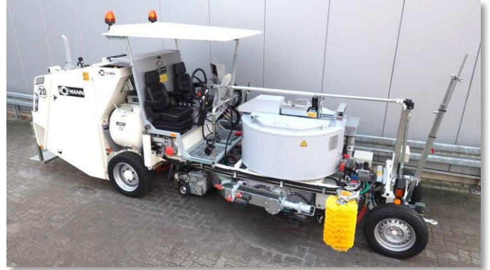
Transport position: Extruder under the container
