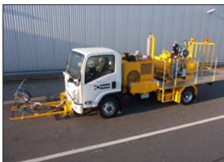
H36-800P in Hong Kong/China with 1-component cold paint Airless system with 90 cm wide line marker unit incl. 4 paint and glass bead guns, 1 x 385 l as well as 2 x 220 l (divided) pressurised containers
