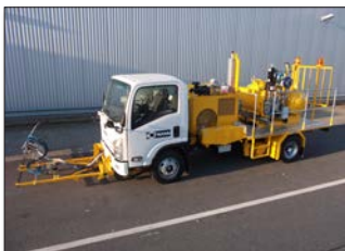
H36-800P in Hong Kong/China with 1-component cold paint Airless system with 90 cm wide line marker unit incl. 4 paint and glass bead guns, 1 x 385 l as well as 2 x 220 l (divided) pressurised containers
