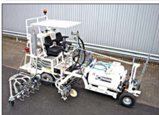
H18 at Royal Air Force/UK equipped with 1-component cold paint Airless system (two pumps) with 90 cm wide line marker unit incl. 4 paint and glass bead guns as well as 3 paint- and glass bead guns for taxiways (black/yellow/black), 2 x 225 l pressurised container
