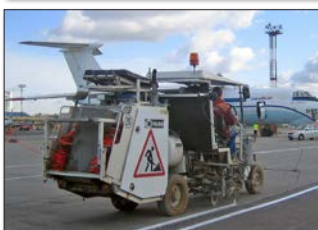
H26 in Saint Petersburg/Russia equipped with 1-component cold paints as well as sprayable 2-component cold plastics Airless system 98:2, 460 lts pressurised container, for use with one paint gun resp. 2-component spray gun for taxiways
